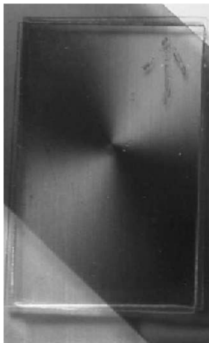
FIGURE 2 The light reflection on the filter when part of the filter (corners) are not covered with the polarising sheet.
